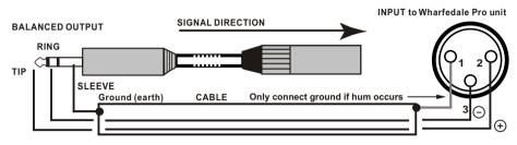
BALANCED INPUT WIRING TO WHARFEDALE PRO UNIT WITH STEREO 1/4" JACK to XLR CONNECTORS
